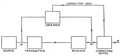
Fig. 8—Schematic diagram of a correction system.
