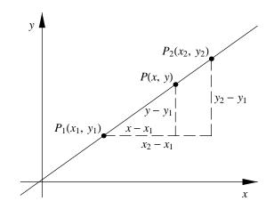
Figure 5.2: Two-point form of a line.
