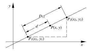
Figure 3.6: Point offset a distance towards a point.
