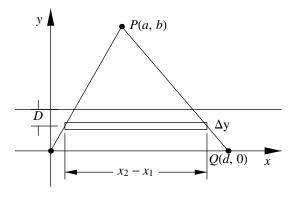
Figure 8.2: Centroid of a triangle.
