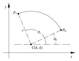
Figure 7.1: Definition of an arc.
