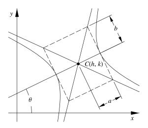
Figure 22.6: Standard representation of a Hyperbola2D.
