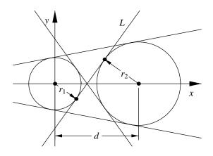
Figure 18.6: Lines tangent to two circles.
