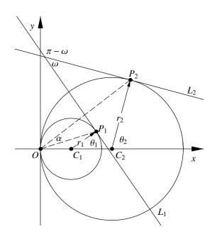
Figure 21.2: Knot point angles.
