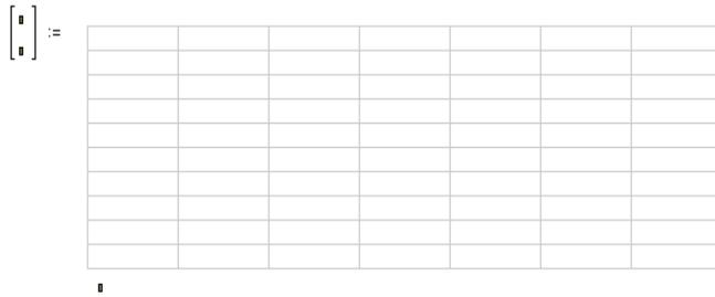
The placeholder(s) at the bottom of the component are for the names of previously defined input variables. The placeholder(s) you see to the left of the := are for the output variables.
