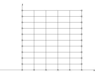
Figure 66: Uniform mesh for the heat equation
