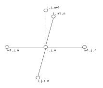
Figure 77: Computational molecule for the explicit solver for 2D heat equation
