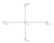
Figure 79: Computational molecule for Laplace's equation
