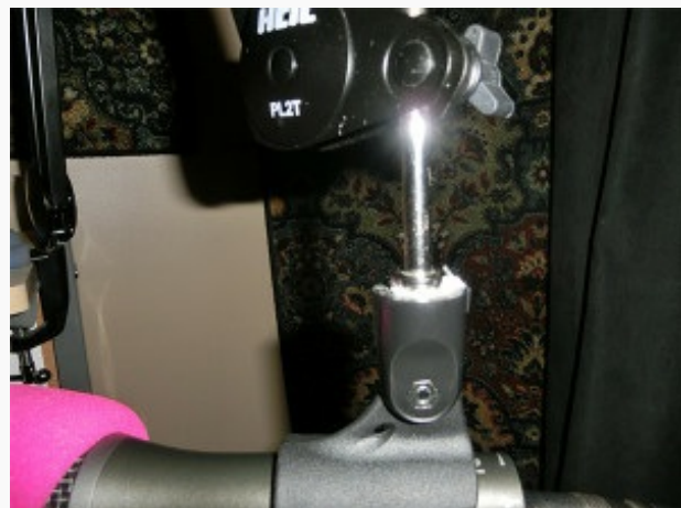
Shims of paper towels in mic clip threads to make a tight fit.
