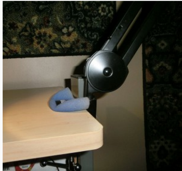
Foam windscreen above and below clamp to transmit less bumping from scissor-mount mic stand
