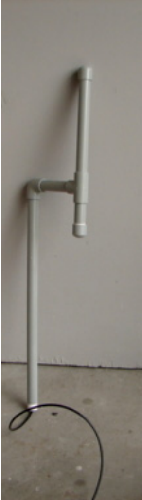
Rubber ducky antenna inside a PVC housing.
